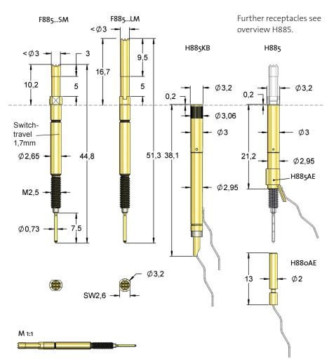
The probe F885 can be height adjusted by 5,0 mm independently from the used receptacle. It is held in its position by pressure marks. For further receptacles see datasheet H885.
