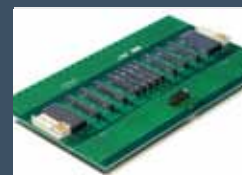
Micro-TCA Backplane Direct Connector for High-Speed Applications up to 12,5 Gbit/s
