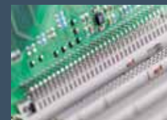
DIN 41612 for robust Signal- and Power-Connections
