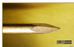
Test probe tip after 10 penetration cycles
