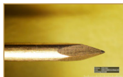
Test probe tip after 5 penetration cycles
