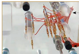
Top contacting with pushrods (NHS)
