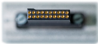
Connector (STK-X,XX) STK-1,27-M-020-Samtec (part 50005 – view from above)
